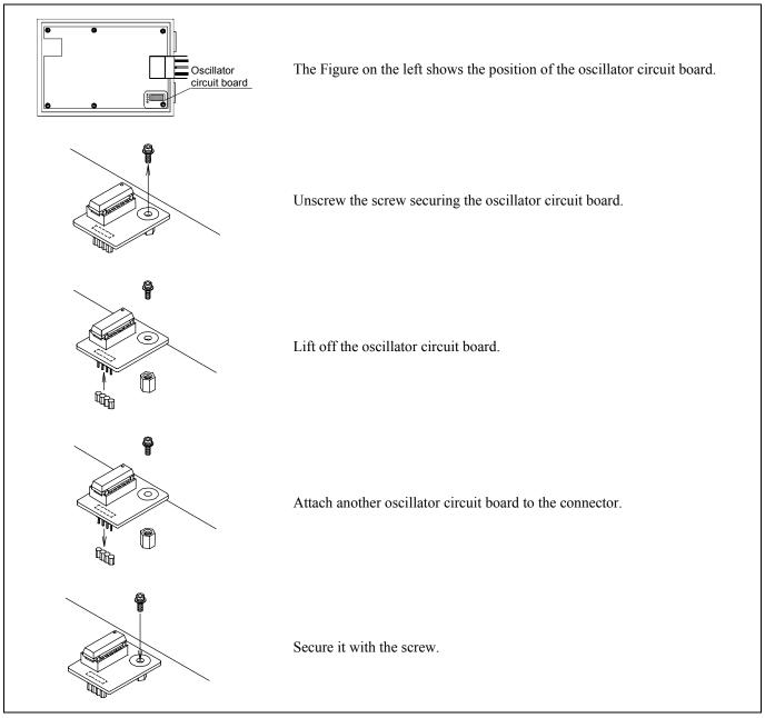
Figure 2.19 Replacing the oscillator circuit board
